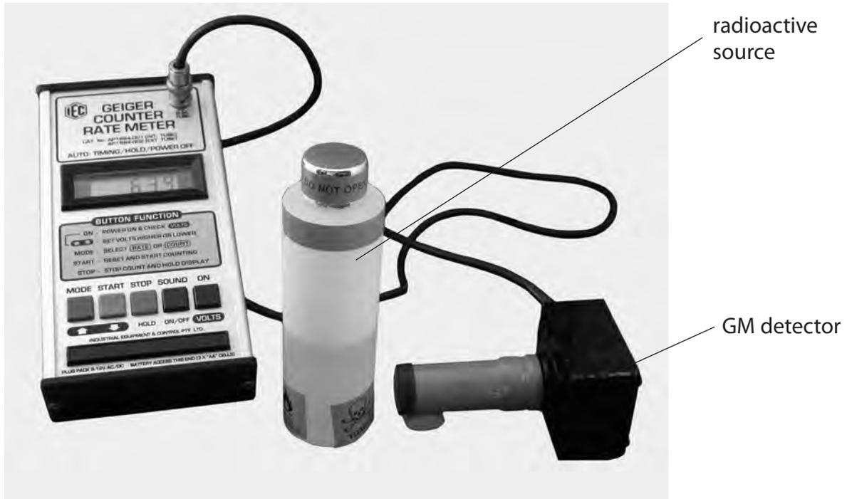
(a) The readings from the counter need to be corrected for background radiation.
